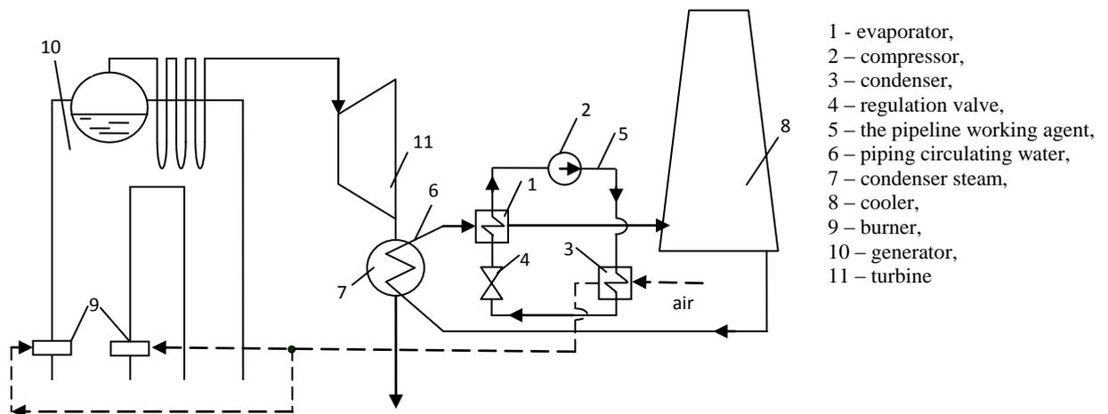
Figure 3 – Basic circuit of heat pump switching on at CHP by utilizing the rejected heat of circulation water
